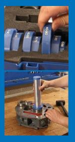
Select the correct collett size and sleeve using the chart above. The bearing must be at a right angle to the shaft. In addition, the shaft should be slightly lubricated.
